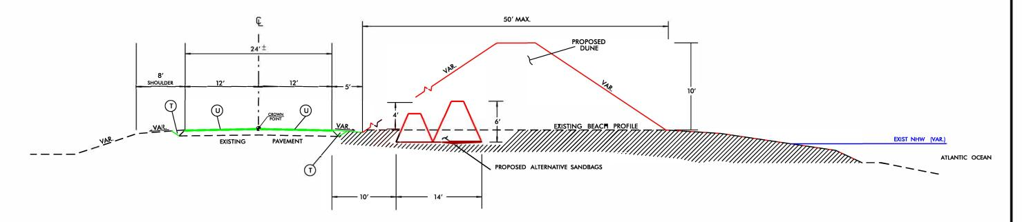
\* MATERIAL USED FOR DUNE CONSTRUCTION AND SAND BAG FILLING SHALL HAVE BEACH QUALITY CHARACTERISTICS AND SHALL BE APPROVED BY THE ENGINEER PRIOR TO PLACEMENT
